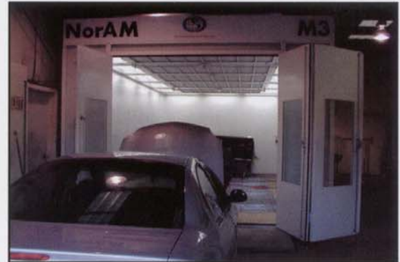
M3 BOOTH WITH UPGRADED 4-ROW PIT AND SURROUND LIGHTING
